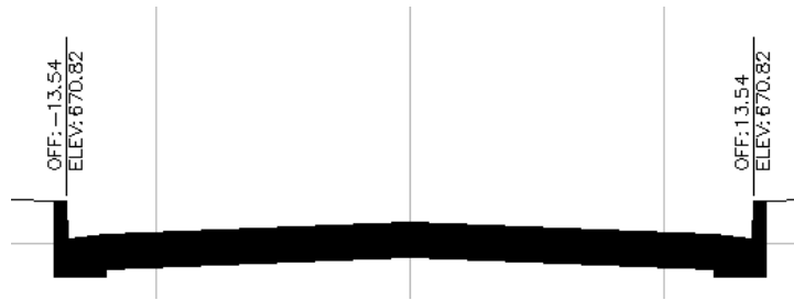
Figure 9. This example shows Top_Curb codes being used to label cross sections. Offsets and elevations are automatically derived from the corridor model and conform to company or jurisdictional CAD standards.
