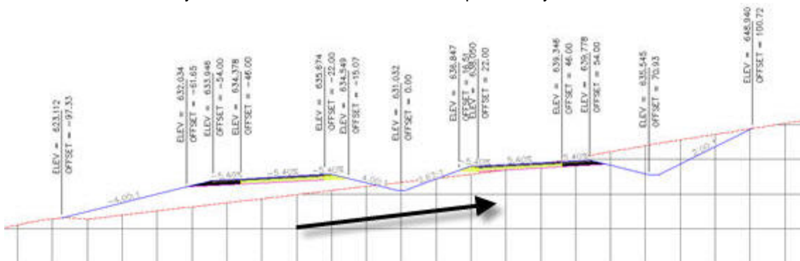
Figure 18. In the example above, the LaneOutsideSuper subassembly is using data from the Outside Lane column, in the Alignment properties.
