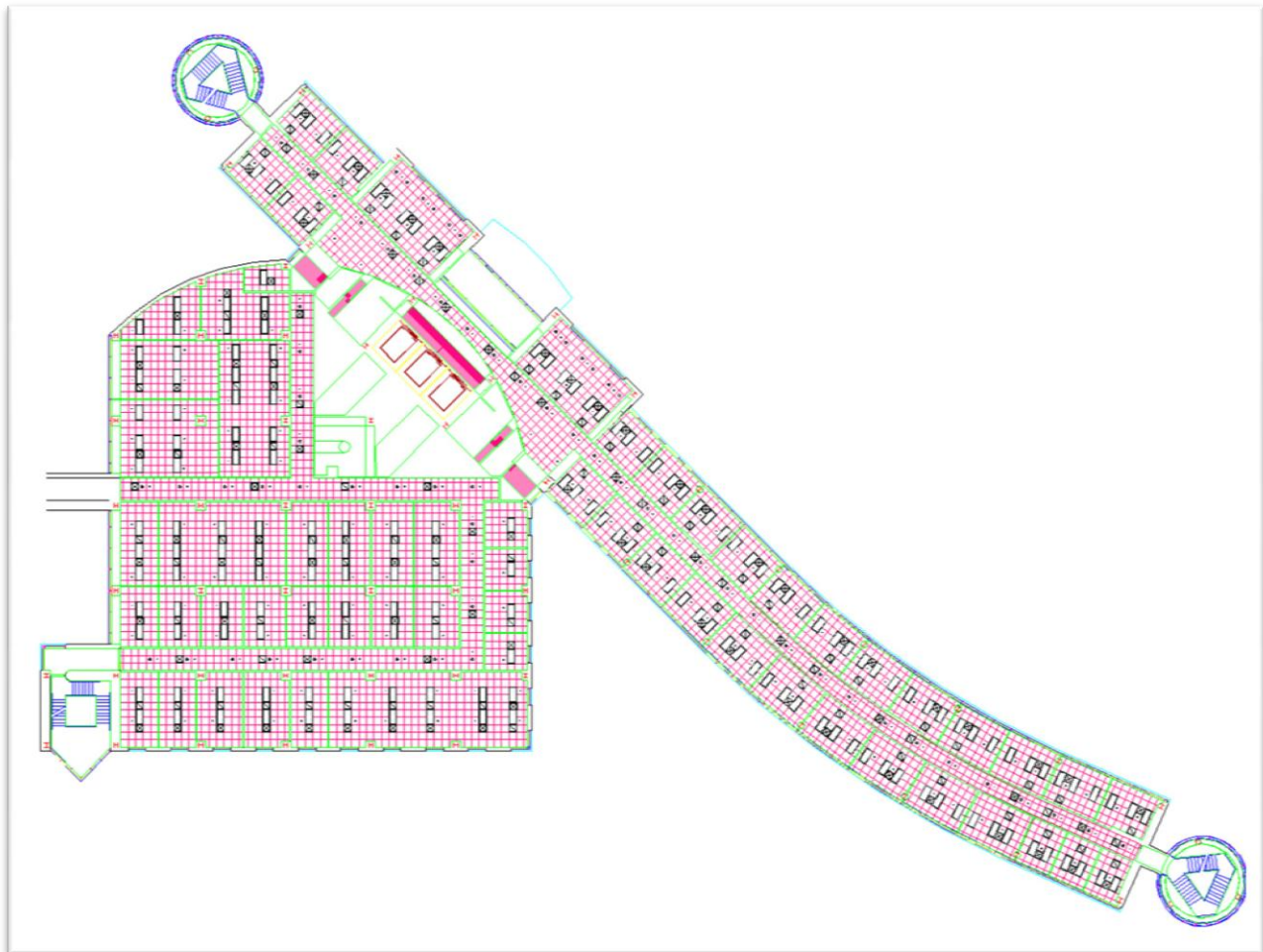
Figure 4: Completed task #4 drawing – a reflected ceiling plan of a complex office building.
